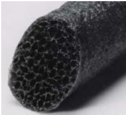
Sample Bead of Closed Cell Foam
