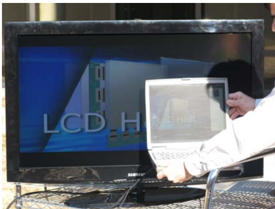
Left: Anti-Reflective glass dry-bonded to 40" LCD TV in direct sunlight. Right: Sunlight readability example – Air gapped vs. Laminated.
