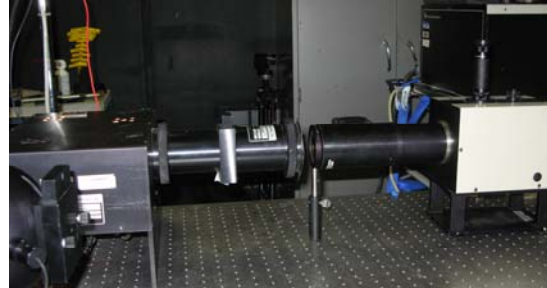
Schematic: Method of measuring internal transmittance. Photo: Internal transmittance test setup.
