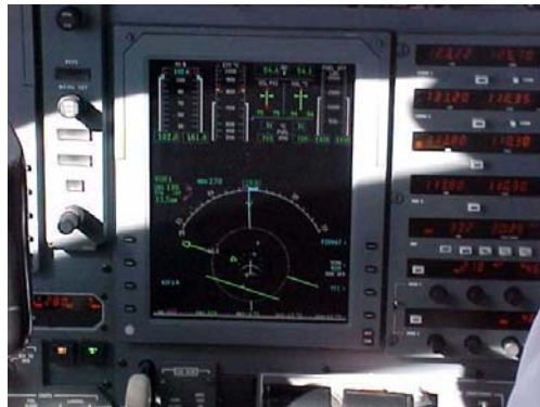
Example of Shafted Sunlight in a cockpit with Laminated Display
