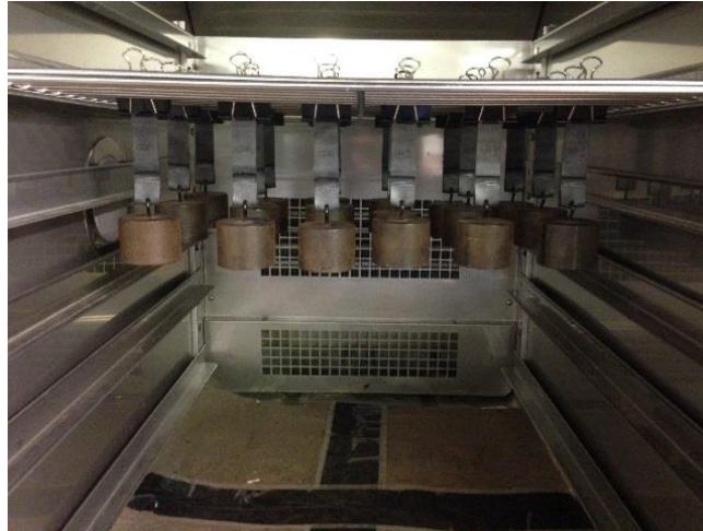
Figure 3 . Shear Adhesion Failure Temperature (SAFT) samples suspended for testing in an environmental chamber.
