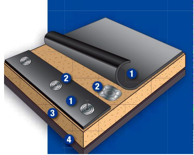
Figure 2. Diagram of a mechanically fastened EPDM roof system showing (1) EPDM membrane, (2) fastener plates, (3) insulation, and (4) roof deck. The tape on the top piece of membrane will create the seam over the three fastener plates in the bottom membrane.
