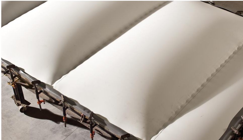
Figure 4. A white mechanically fastened roof undergoing a wind uplift test. The fasteners are visible within the seams. [7]
