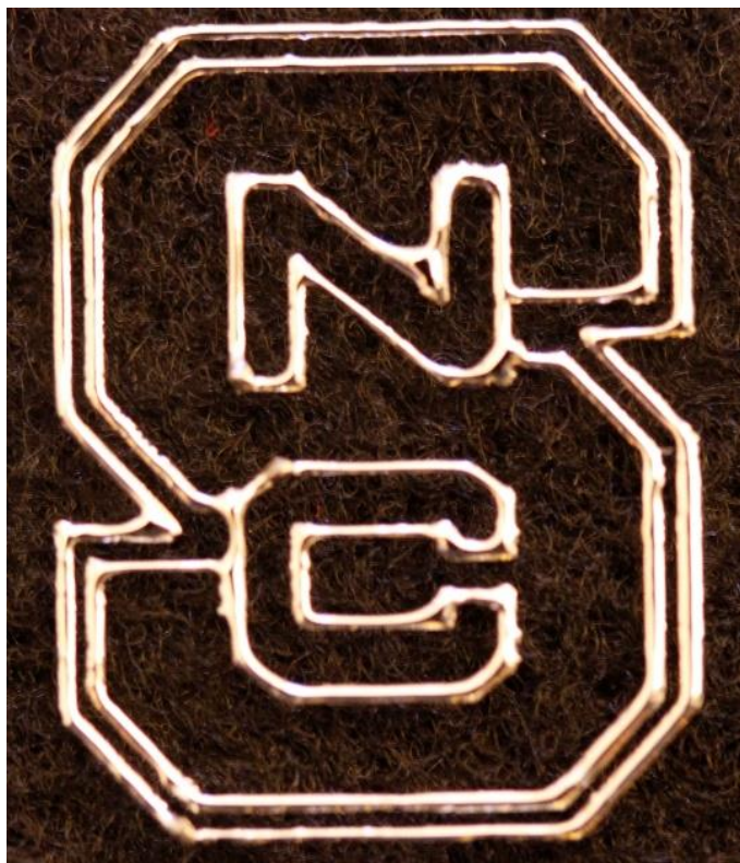
Figure 2. Liquid metal printed in the NC State logo. This shape is maintained solely due to the native oxide that helps preserve the shape and adhere the metal to the surface.
