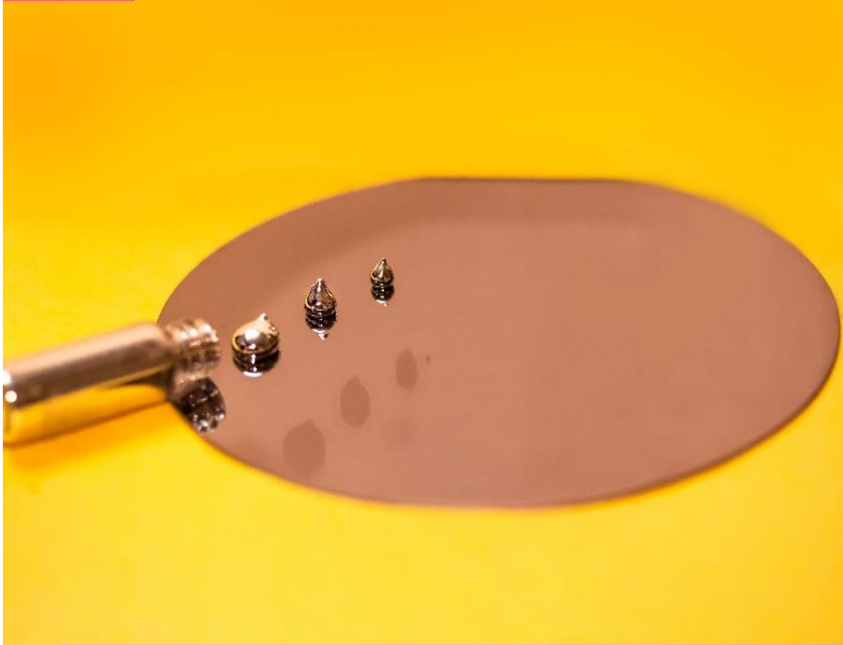
Figure 1. (Left) Droplets of liquid metal maintain non-spherical shapes due to the presence of the nm-thick oxide layer. Normally, droplets of liquid would assume spherical shapes due to surface tension.
