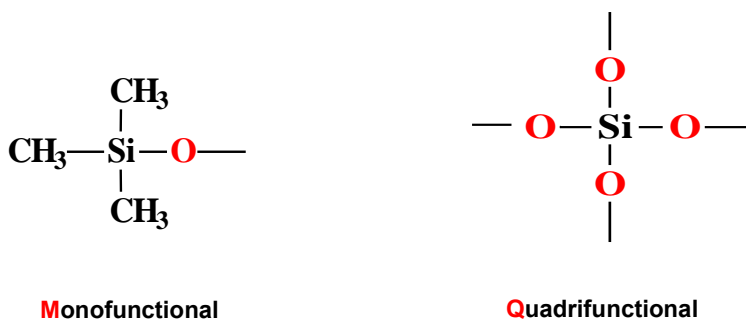
Figure 2. Typical Structure of M unit & Q unit
